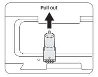
3. Pull out the halogen lamp from the holder and replace it. To assemble halogen lamp, proceed opposite order from above instructions.
