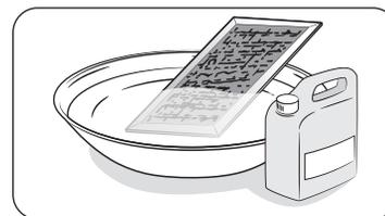
3. Soak the grease filter in hot water mixed with a mild detergent. Rinse well and shake to dry. If necessary, brush the filter lightly to remove embedded dirt.
