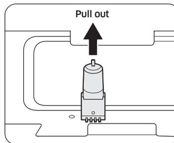
3. Pull out the halogen lamp from the holder and replace it. To assemble halogen lamp, proceed opposite order from above instructions.
