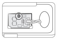
3. Remove the screw securing the LED lamp board.
