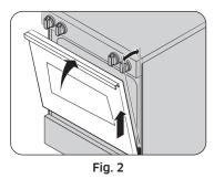
**5.** Lift door up and out until the hinge arm is clear of the slot (Fig. 2).
