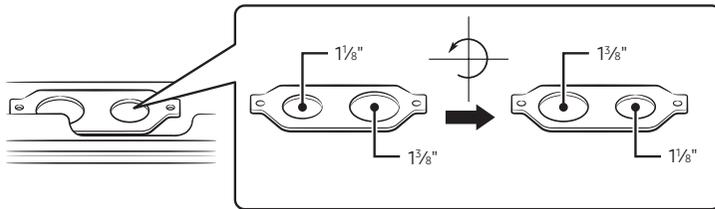
Remove the conduit connection plate and rotate it as shown below.
