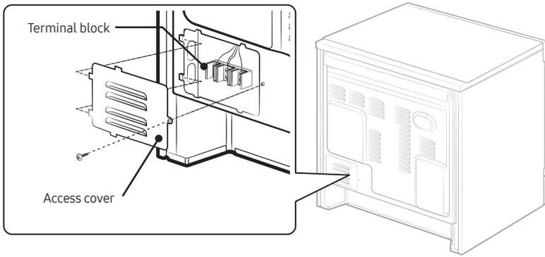
Loosen and then remove the rear access cover screw with a screwdriver. Remove the rear access cover by pull right and then out. The terminal block will then be accessible.
