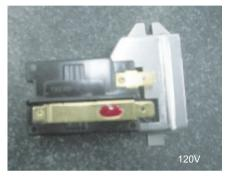
**Igniter(101D)** Resistance value 40~400 Ω If resistance is infinite, replace Igniter
