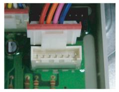
**Sensor Bars** - Disconnect harness and test Pink wire Pin 4 to Orange wire Pin 5. Approx  $\infty \Omega$  without laundry Approx 190 $\Omega \pm 10\%$  with wet clothes
