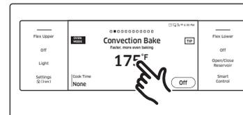
Tap the temperature area, enter the new temperature using the numeric keypad and then tap **OK**.
