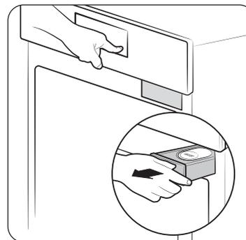
1. Locate the water reservoir. The water reservoir is on the right side of the oven, just above the oven opening. Touch **Open/Close Reservoir** on the control panel to eject the water reservoir. Grab the front of the reservoir, and then slide it out to remove.
