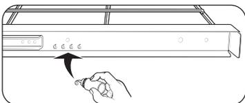
4. Shake the graphite lubricant before opening it. Starting with the left (front and back) slide mechanism of the rack, place four (4) small drops of lubricant on the two (2) bottom tracks of the slide close to the bearing carriers.
