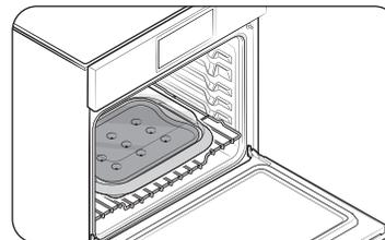
4. Push the container in until the steam nozzle enters the hole on the convection fan cover.
