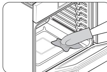
6. Clean the oven's interior. There will be a significant amount of water remaining on the bottom of the oven after a steam-cleaning cycle. Remove the residual water with a sponge or soft dry cloth.
