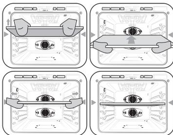
1. Insert the divider into the 4th rack position of the cavity.
