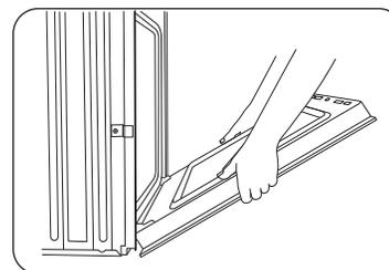
5. Partially close the door to engage the door latch locks. The door will stop at this point.
