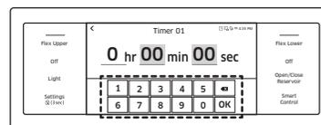
4. Tap the numbers on the numeric pad to set the time. (You can set the timer for any amount of time from 1 sec to 99 hr 59 min 59 sec).
