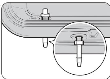
2. Insert the steam nozzle to the hole on the right-rear side of the metal pan, and then tighten the provided nut.
