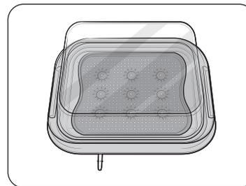
3. Put the steam tray in the metal pan, and then close the glass lid to use it in the oven.
