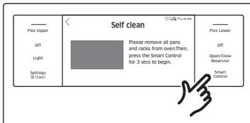
9. Press the **Smart Control** for 3 secs to begin self-cleaning. The motor-driven door lock will engage automatically.
