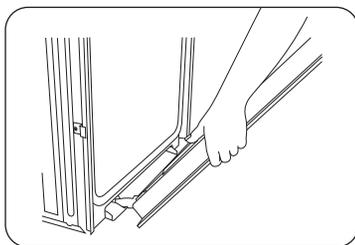
1. Using two hands, grasp the side edges of the door at the midpoint. Face the oven cavity.
