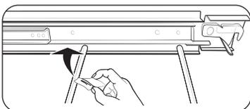
3. If there is debris in the slide tracks, wipe it away using a paper towel. (Any graphite lubricant wiped away must be replaced - See steps 4 through 7).
