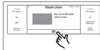
4. Pour approximately 10 oz. (300 ml) of water onto the bottom of the empty oven and then close the oven door. Use normal water only, not distilled water. Tap **OK** to begin steam-cleaning. The motor-driven door lock will engage automatically.
