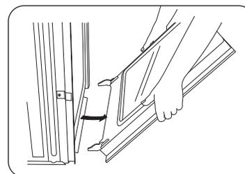
6. Using two hands, grasp the edges of the oven door. Lift and pull the oven door toward you and remove. You may need to gently shift the door from side to side as you pull.
