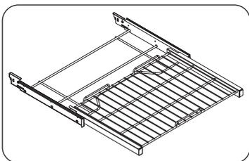
1. Remove the rack from the oven. See removing the gliding rack in the **Using the gliding rack** section on page 49.
