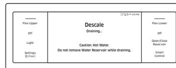
5. When descaling is complete, the oven drains water automatically.
