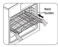
With the Gliding rack in the Closed position and the oven off, carefully insert the Gliding Rack between the guides until the rack reaches the back.
