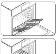
1. Place the end of the wire rack steam on the support.
