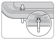
Insert the steam nozzle to the hole on the right-rear side of the metal pan, and then tighten the provided nut.
