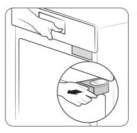
Locate the water reservoir. The water reservoir is on the right side of the oven, just above the oven opening. Touch Open/ Close Reservoir on the control panel to eject the water reservoir. Grab the front of the reservoir, and then slide it out to remove.
