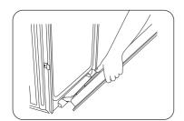
Hold the door at a 45 ° angle, and then 3. align the door hinges with the slots in the lower front of the oven cavity. Slowly insert the door, making sure you maintain the 45 ° angle. You will know the door is engaged in the slot when you feel a slight drop.
