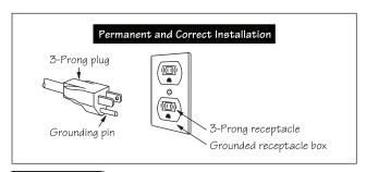
**AWARNING** Improper use of the grounding plug can result in a risk of electric shock. Do not use an extension cord. If the power supply cord is too short, have a qualified electrician or serviceman install an outlet near the appliance.
