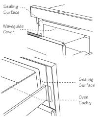
**2** Remove the feature sticker, if there is one. Check the drawer for any damage, such as misaligned or bent
