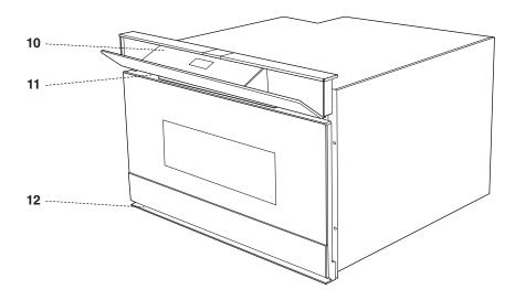
The keysheet is hidden behind the control panel door on the top front face of the unit. To open, push in on the control panel The panel will release and gently float to open. To close, push the panel upward to the closed position. The panel will be secured by magnetic latches in both open and closed positions.
