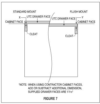
7. Slide the unit into the opening. Plug oven into the wall receptacle prior to pushing the unit all the way in. See Figure 8. The mounting angles of the oven should rest against the installed wooden cleats.
