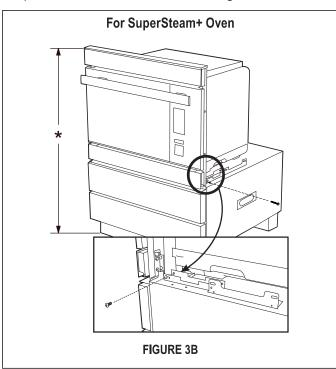
4. Adjust the height of the overall unit to fit your specific opening. The pedestal contains 4 adjustable feet. To adjust, have one person tilt the unit to one side while the other person adjusts the 2 feet on the raised side to the desired height. Repeat this step by tilting the unit to the other side and adjusting the other 2 feet. Ensure that all feet are adjusted equally to balance the unit. See Figure 4.
