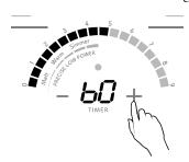
**3** Use the Power Slider Bar selector to set power level.
