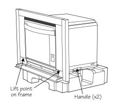
Remove all packing material. Review installation instructions. Lower drip tray door and lift from these points for installation.
