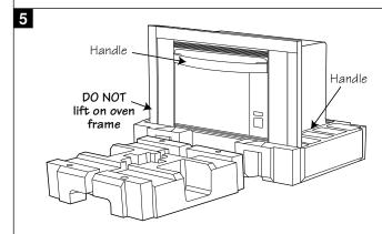
Carefully lift from front handle and lower center back of oven.
