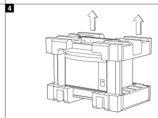
Remove top foam packing and place in front of the unit as shown in figure 5.
