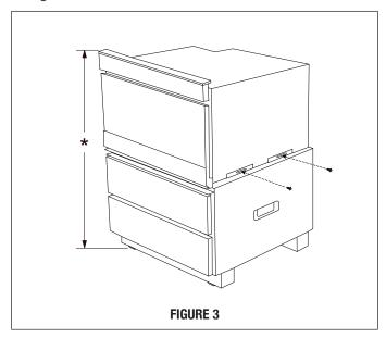
4. Adjust the height of the overall unit to fit your specific opening. The pedestal contains 4 adjustable feet. To adjust, have one person tilt the unit to one side while the other person adjusts the 2 feet on the raised side to the desired height. Repeat this step by tilting the unit to the other side and adjusting the other 2 feet. Ensure that all feet are adjusted equally to balance the unit. See Figure 4.
