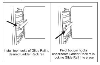
**3** Ensure the Glide Rails are level on each side of the wall. Place the oven rack or drip pan onto the Glide Rail. The rack should now slide freely.
