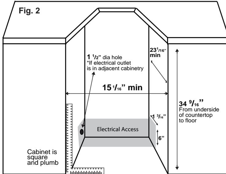
Important: The listed depth requirement for the installation is assuming that the electrical outlet is located in the adjacent cabinetry or is flush mounted in the rear wall, not surface mounted in the enclosure.
