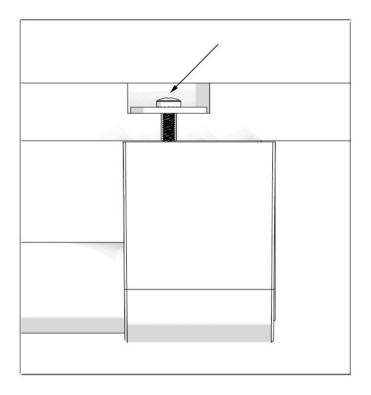
• Use 4 screws to group the freezer inner door on the furniture door as shown in the figure below.
