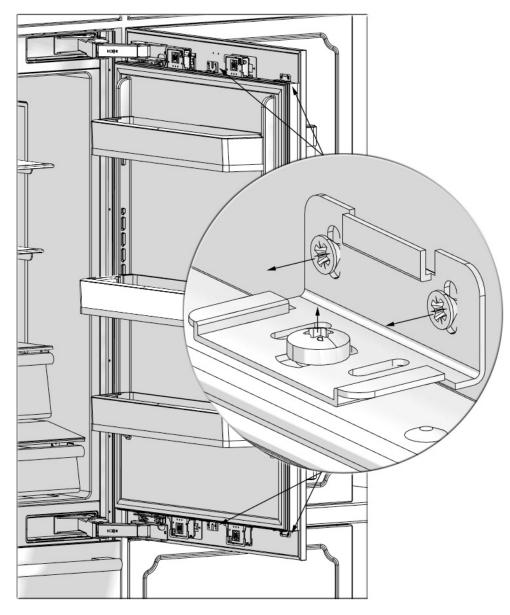
• Remove the screw of FF Upper and Lower mechanisms.
