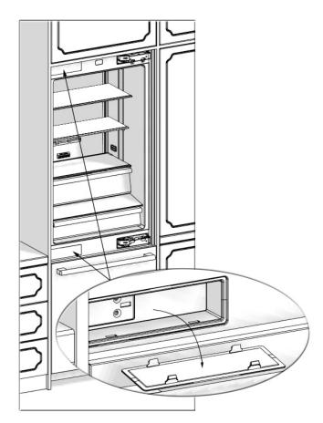
• Remove the Screw caps of the hinges.
