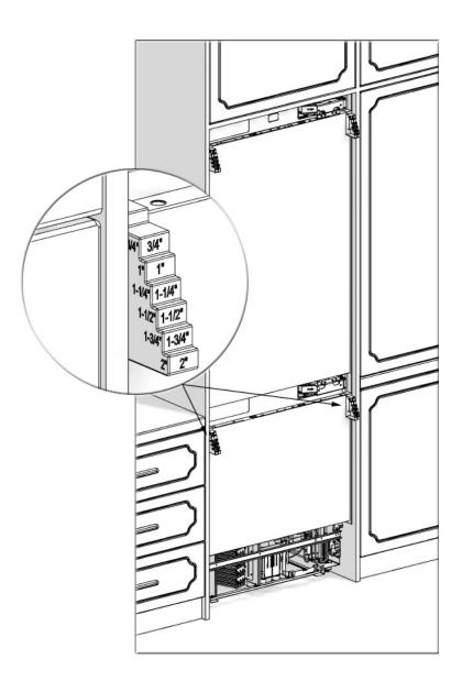
• Position of the level adjustment part (10) must be adjusted according to the thickness of the door. It can adjust the level for 6 different door thickness levels.
