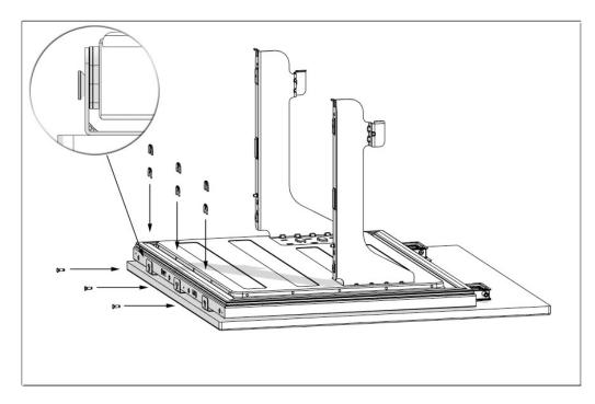
A total of 3 mm washers must be placed on the FRZ Door (2+1) on the condition that all furniture dimensions are suitable. Washers to be used are determined based on the kitchen design.
