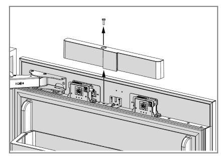
• Loosen one screw of the Lower Cover of the Fridge Door and remove it.
