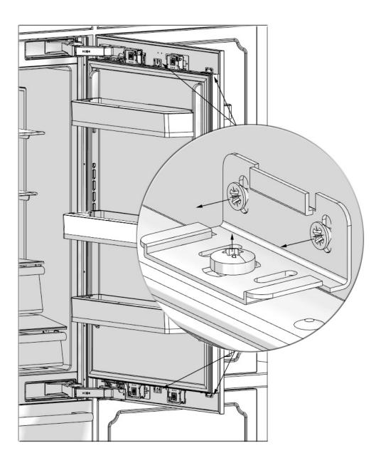
• Loosen 3 bracket screws at the upper section of the freezer door.
