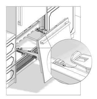
• Fix the Freezer Furniture door assembly onto the rails with 2 screws.
