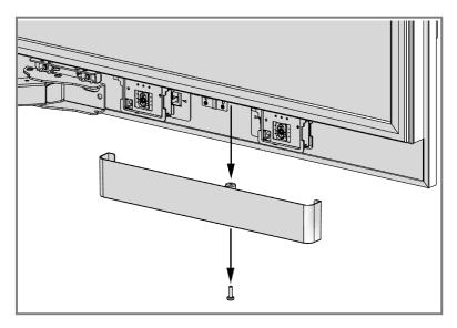
• Remove FF Lower and Upper Bracket screws.
