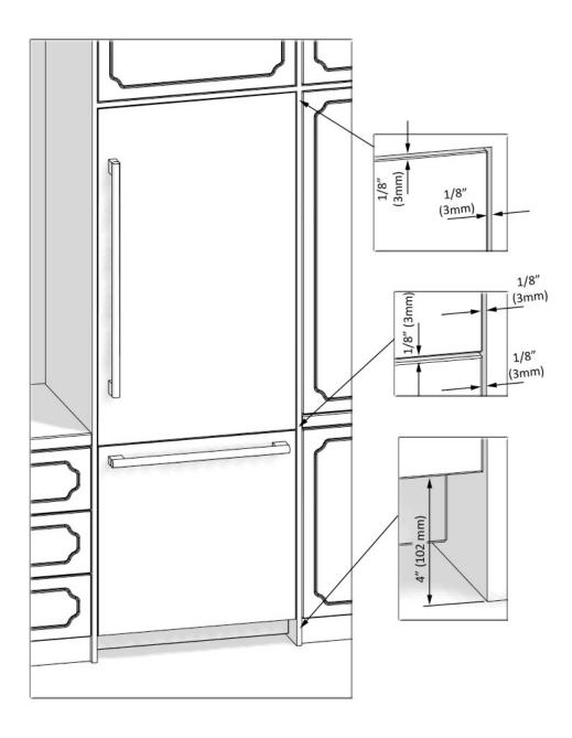
• Adjust the Furniture Doors with the 3D adjusting mechanism.
