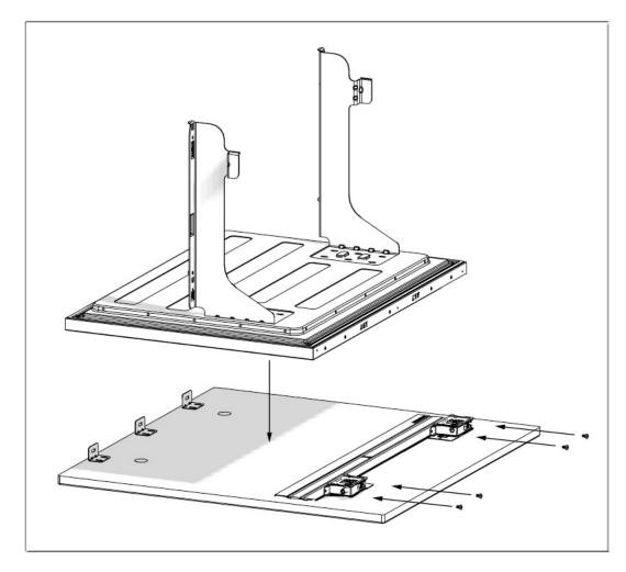
• Attach the brackets to the freezer inner door, using 1 bolt (27) for each bracket and the Crescent Washers (12) specified below.
