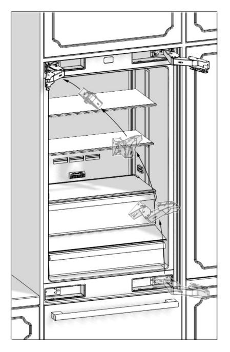
• Remove the upper right hinge by loosening its 2 screws and fix it to its slot at the lower Left side.
