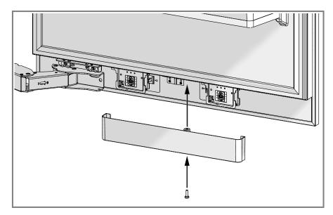
• Attach the FRZ Cover (6) using the tabs.
