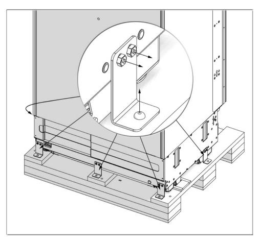
• ove the screws that hold the rear foot of the Wooden Pallet.
