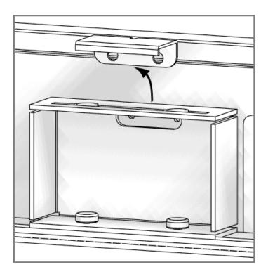
• Remove 2 screws of the Hanger Carrier.
