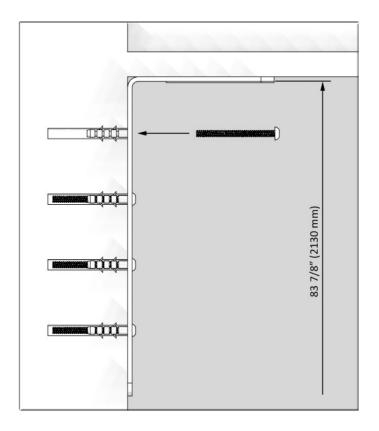
If there is furniture at the back wall of the refrigerator, please make sure that the furniture is fixed to the wall. For this, you need to be sure that the back wall of the furniture is fixed to the concrete back wall with suitable connection parts
