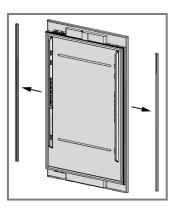
• Loosen one screw of the Upper Cover of the Fridge Door and remove it.
