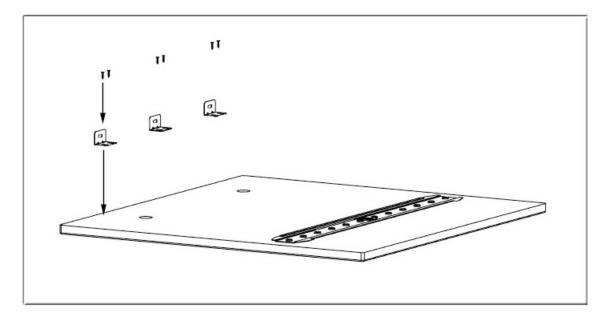
• Attach the 3D adjusting mechanisms you have removed from the door to the door cradles.
