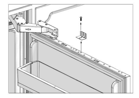
• Attach the FF Hanger Bracket (13) part in the mounting box to its place with the help of 2 screws (16).
