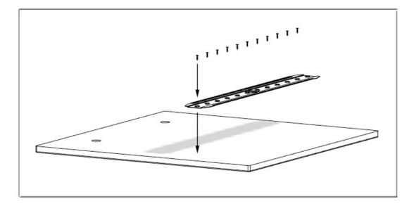
• Attach 3 sheet metal brackets (25) using 2 screws (26) for each.
