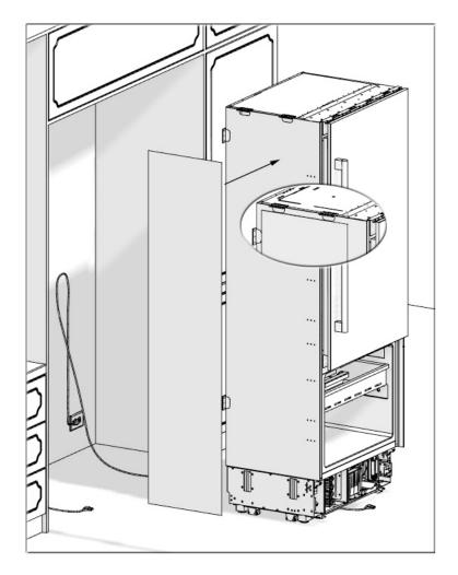
• Bring the two refrigerators side by side. After making sure that they are in alignment, screw the fasteners (33) to the other refrigerator.
