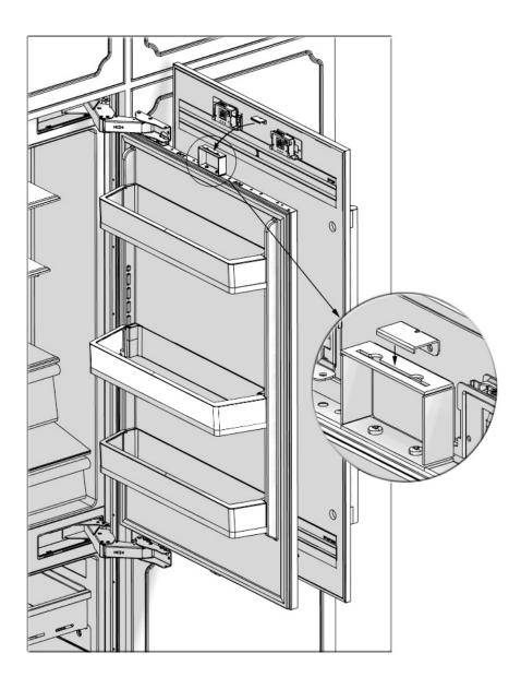
• Group the FF Upper Mechanism with 4 screws.
