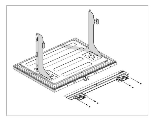
• Take out the cradle parts from the mechanism assemblies.
