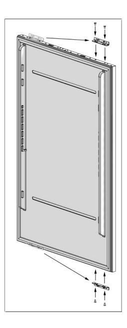
• Attach the Hanger Sheet (13) using 2 screws (16).
