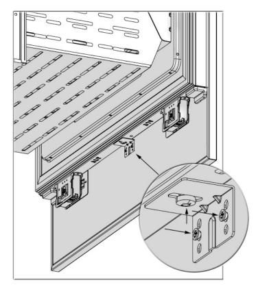
• Attach the lower side brackets of the Freezer Door.
