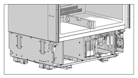
• After adjusting the adjustable feet, check the flatness in both width and depth directions.
