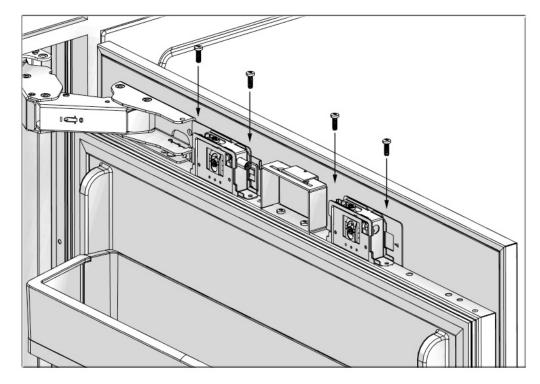
• Group the Lower Mechanism with 4 screws.
