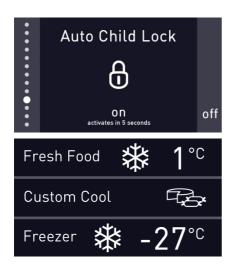
The child lock page is a feature for preventing children from changing the product settings. A lock symbol will appear on the display and the lock will be enabled 5 seconds after you have pressed "on" key on the child lock page. Buttons are inactive when this function is enabled. When you press any key to deactivate the lock, you will see "Cancel child lock?" on the display. You can exit this mode by pressing "Yes".
