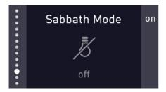
This product has a Sabbath feature. Lights of the refrigerator will not become on, the display will not operate and the door open alarm cannot be activated while the Sabbath mode is active. You can use "On" or "Off" features to activate/deactivate this mode.
