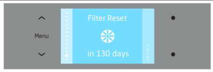
The filter counter is activated with the buzzer sound. After 130 days, the display shows a filter change warning. After the filter is replaced with a new filter, pressing the reset button on the Filter Reset page starts to count down to 130 days. To cancel this function, please press the reset button again.
