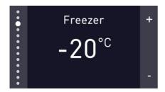
It allows you to set the temperature of the freezer compartment. You can use "+" and "-" keys to set the temperature of the freezer compartment to -18, -19, -20, -21, -22, -23, -24 °C (0, -1, -2, -3, -4, -5, -6, -7, -8, -9, -10, -11, -12°F) respectively.
