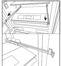
2. Place the gap at the rear corners of the crisper to the detail located at the rear section of the rails.
