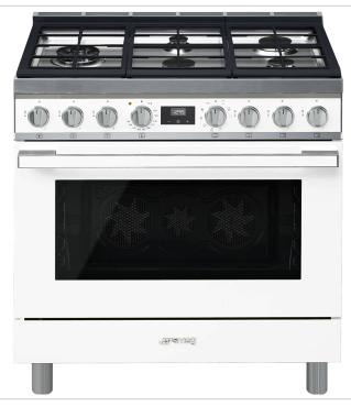
• Rangetop • 5 cooking zones • Full-width continuous grates • Left double-inset super burner: up to 18,000BTUs • Oven • 10 cooking functions • Oven capacity: 4.5 cu.ft. • Ever Clean enamel • 5 shelves • Tilting grill • 3 fans • 2 halogen lamps • Oven door with 3 layers of glass • Full-glass internal door • Removable internal glass panel • Silent Close door closure • Programmable timer • Cooking start time and end time programming options • Cooling fan system • Push-pull storage
