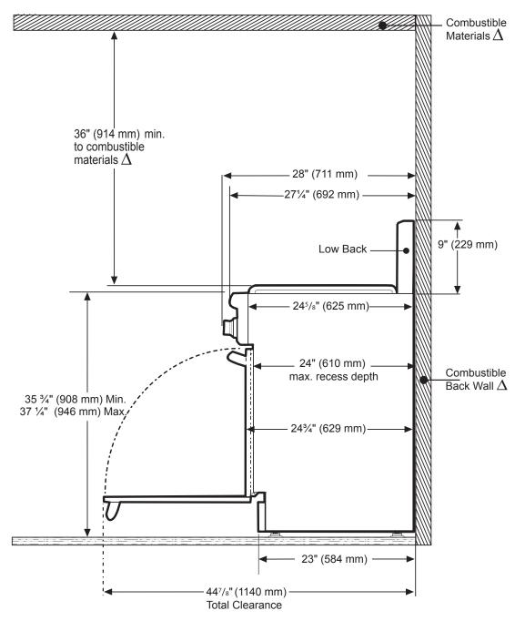
$\underline{\Lambda}$  As defined in the "National Fuel Gas Code" (ANSI Z223.1, Current Edition). Clearances from non-combustible materials are not part of the ANSI Z21.1 scope and are not certified by CSA. Clearances of less than 12" (305 mm) must be approved by the local codes and/or by the local authority having jurisdiction.
