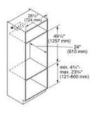
Junction box may be installed above, below, or to the right of the unit within range of the power cable.
