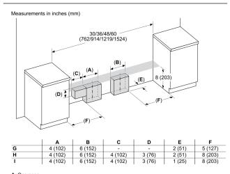
A: Gas zone B: Electric zone G: All Harmony series H: 36"/48" Grand series I: 60" Grand series Measurements in inches (mm) 23/<sub>16</sub> (55) 27<sup>3</sup>/<sub>16</sub> 29<sup>15</sup>/<sub>16</sub>/35<sup>15</sup>/<sub>16</sub> (760/913) 24<sup>7</sup>/<sub>16</sub> (691) (621) <sup>3</sup>/<sub>4</sub> ↓ (19) ↓ 24<sup>3</sup>/<sub>4</sub> (630) 353/4-363/4  $27^{3}/_{8}$ (908 - 933)(695) 53/4 22<sup>5</sup>/<sub>8</sub> (575) (147)447/8 Α  $(1140)_{\sim}$ 2<sup>5</sup>/<sub>8</sub> (67)
