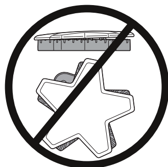
Incorrect burner cap
