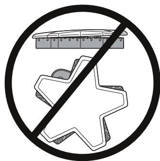
Incorrect burner cap
