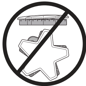
Incorrect burner cap
