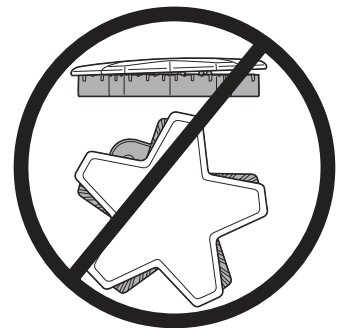
Incorrect burner cap
