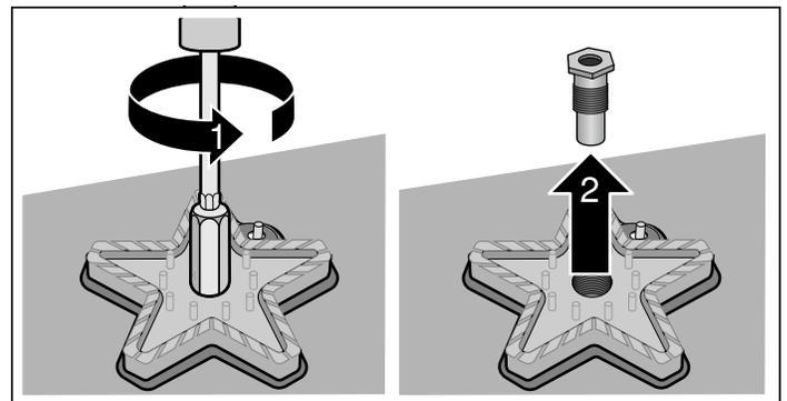
3. Set the NG (natural gas) venturis aside, noting from which burner they were removed, and save for later use if necessary.
