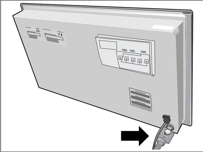
1. Remove the hexagon shaped cap from the regulator making sure not to dislodge the gasket on the cap or the spring inside the regulator.
