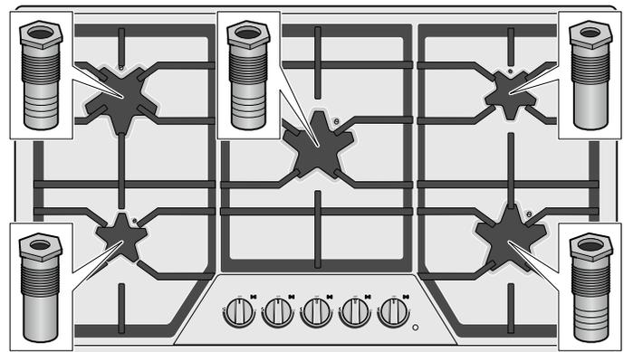
The orifice sizes are shown in the white circles corresponding to each burner as shown in the image above. These numbers are engraved on the side of each orifice. It is very important to install the correct orifice size for each burner.
