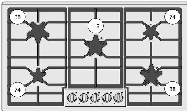
7. Identify the correct placement of the LP gas venturis as layed out in the image below.
