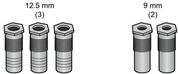
**Note:** Depending on the model, the kit may contain more venturis and orifices than are necessary to complete your appliance conversion.
