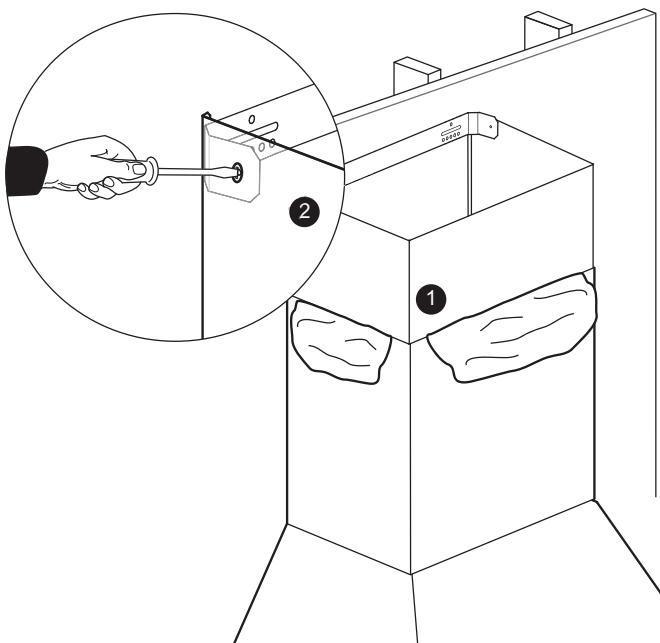
7. From inside of hood, screw the supplied 5/8" (16 mm) sheet metal screws through the holes on each side and along the front into bottom of the extension. Screw quantity is dependent on hood size.
