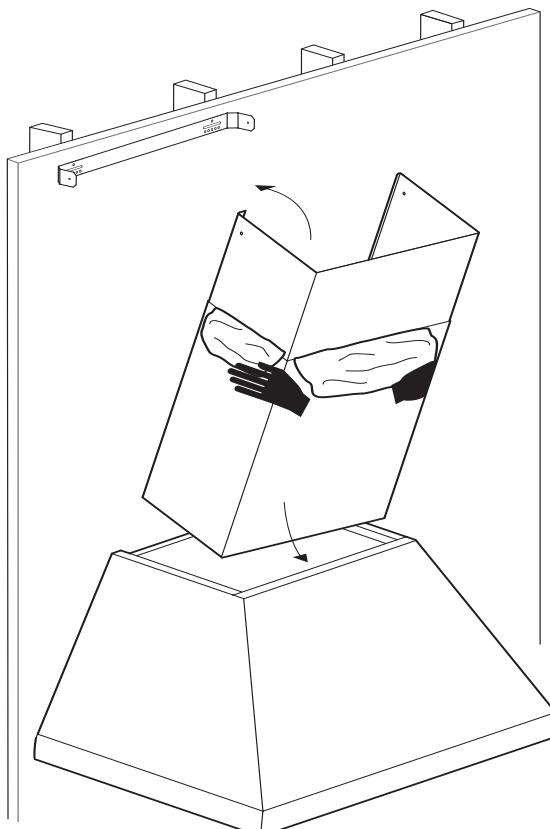
6. Carefully pull the top part of the extension upwards. Screw the left and right sides of the extension to the mounting bracket with the supplied stainless screws.
