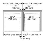
in combination, a minimum distance between the ovens the oven installation measurements.
