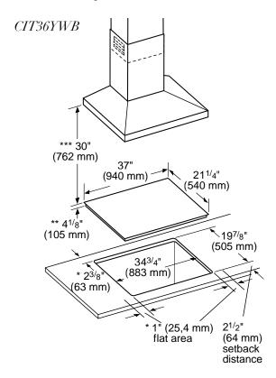
**NOTE:** The work surface should be horizontal and level. The stability of the countertop should be confirmed even after making the cutout.
