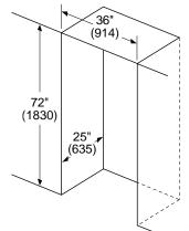
Leave ½" (12.7) gap at the top and 1" (25.4) behind the refrigerator for proper ventilation.
