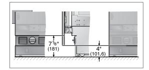
If required by the surrounding cabinetry design, the distance between the bottom edge of the door panel and the floor can be increased from approx. 4" (102 mm) up to 7 1/8" (181 mm), but should not be decreased. Note, however, that the venting grille and (if applicable) water filter cavity will be visible, even if the door is closed.
