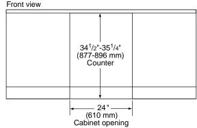
Thermador double drawer under counter top dimension. (Unit door flushed with the cutout) measurements in inches (mm) measurements in inches (mm)
