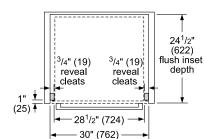
29<sup>1</sup>/8" reveal cleats (740)24<sup>5</sup>/8" (625) cut out measurements in inches (mm)
