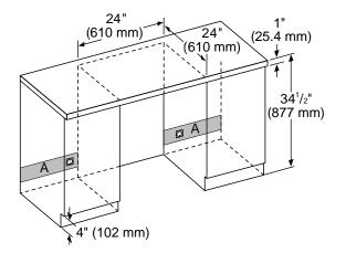
Recommended area for installation connection - a 2<sup>1</sup>/<sub>2</sub>" (63 mm) diameter hole is recommended. Location of power cord at base of the appliance.
