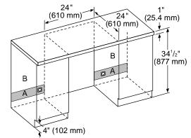
Recommended area for installation connection - a 2<sup>1</sup>/2" (63 mm) diameter hole is recommended. Location of power cord at base of the appliance
