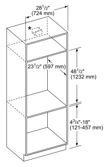
\* Junction box may be installed above, beneath, right or left of the unit within range of the power cord.
