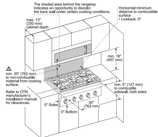
**NOTE:** See the Ventilation Planning Guide for recommended hood options. Due to the high heat of the burners, installing a microwave oven with a ventilation system over the appliance is not recommended on anything other than the 30" 5-Burner. Refer to the OTR manufacturer's installation manual for clearances.
