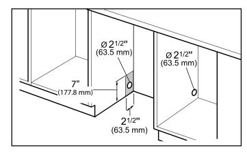
**NOTE:** Plumbing installations will vary — refer to local codes. The maximum length of the drain hose, including hose leading to air gap (if any) is 150" (380 cm). Ensure a portion of the drain hose is raised at least 33" (84 cm) above the floor to ensure proper draining.
