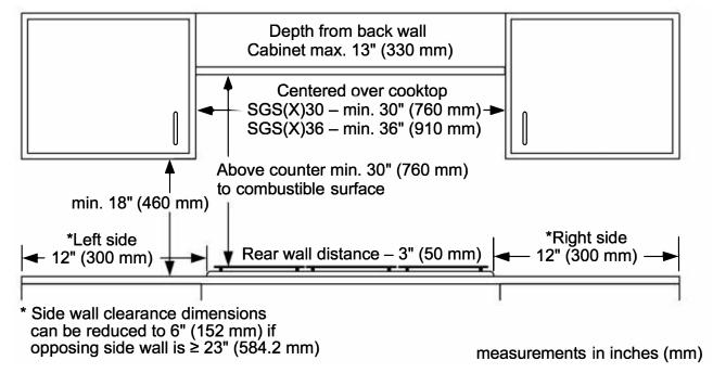
NOTE: Dimension requirements are for combustible surfaces. When the surface is protected by a material listed by UL as a Floor Protector and Wall Shield covered with not less than No. 28 MSG sheet metal 0.015 inch (0.38 mm) stainless steel, 0.024 inch (0.6 mm) aluminum or copper, it is considered noncombustible and some dimensions may be reduced. For a noncombustible surface over the cooktop, the minimum clearance is 24" (61 cm) rather than 30" (76 cm).
