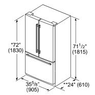
\*Add 5/8" (17) with front leveling feet fully extended \*\* Add 1" (25) for fixed spacers on back
