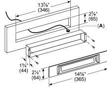
A: DBus Cable length: 30 feet (9180 mm)
