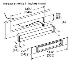
A: DBus Cable length: 30 feet (9180 mm)
