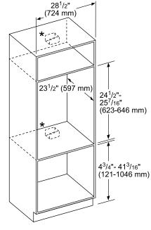
\* For single ovens installed into a wall cabinet, the junction box may be located above, beneath left or right of the unit within range of the power cord
