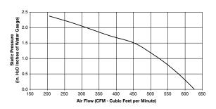
NOTE: All measurements are made with at least 2 ft. of straight length ducting. These are NOT free blowing measurements.
