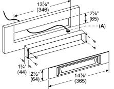
A: DBus Cable length: 30 feet (9180 mm)
