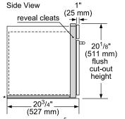
\* Flush installation requires a 5/16" (8 mm) high x 28<sup>1</sup>/<sub>2</sub>" (724 mm) wide x 19<sup>3</sup>/<sub>4</sub>" (500 mm) deep baseplate underneath the unit body.
