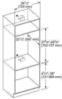
For single ovens installed into a wall cabinet, the junction box may be located above, beneath, left or right of the unit within reach of the power cord.
