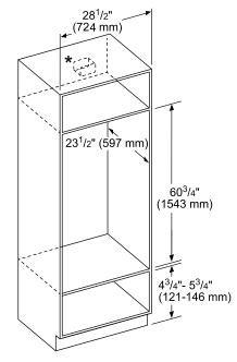
\* Junction box may be installed above, right or left of the unit within range of the power cord.
