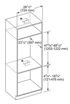
f Junction box may be installed above, beneath, right or left of the unit within reach of the power cord.
