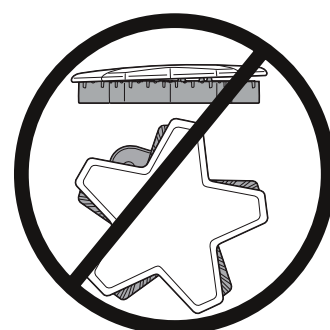
Incorrect burner cap
