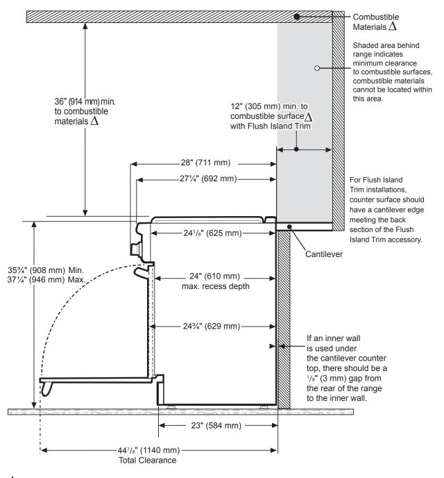
$\Delta$  As defined in the "National Fuel Gas Code" (ANSI Z223.1, Current Edition). Clearances from non-combustible materials are not part of the ANSI Z21.1 scope and are not certified by CSA. Clearances of less than 12" (305 mm) must be approved by the local codes and/or by the local authority having jurisdiction.
