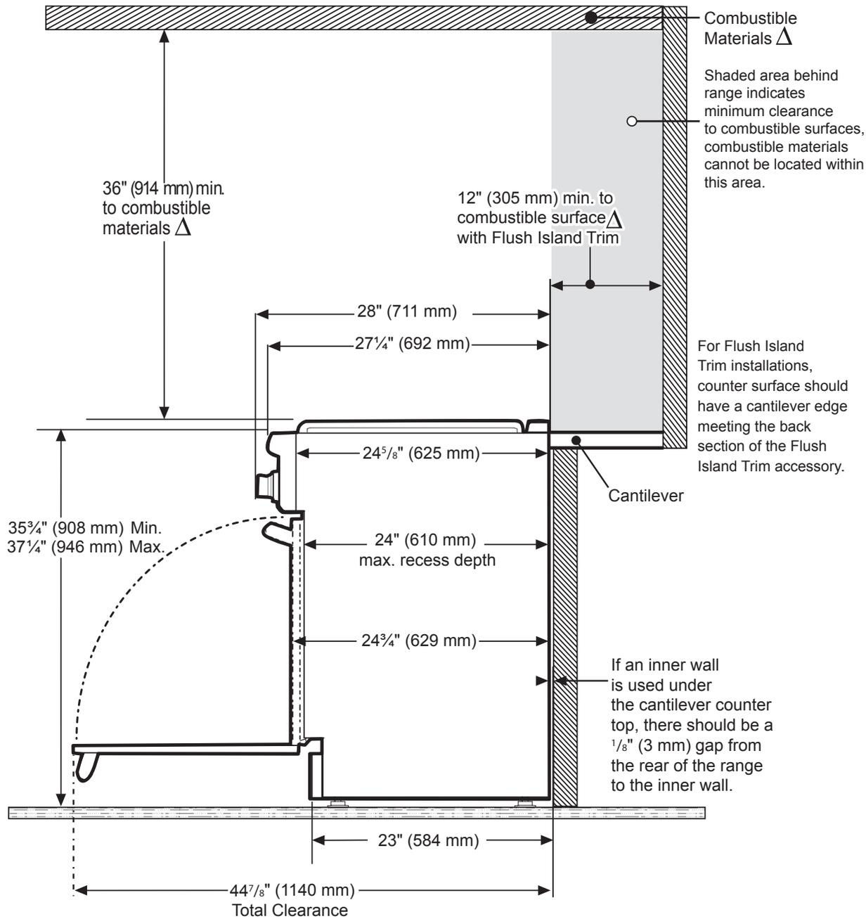
△ As defined in the "National Fuel Gas Code" (ANSI Z223.1, Current Edition). Clearances from non-combustible materials are not part of the ANSI Z21.1 scope and are not certified by CSA. Clearances of less than 12" (305 mm) must be approved by the local codes and/or by the local authority having jurisdiction.
