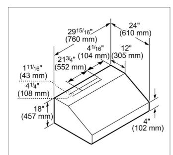
measurements in inches and mm
