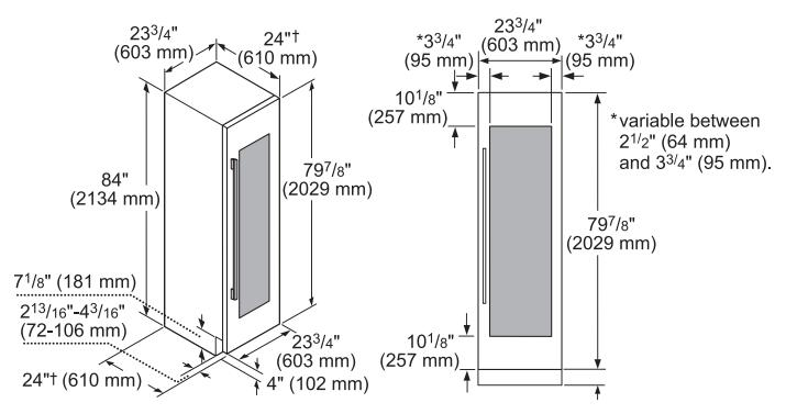
†Excludes thickness of door panel. If standard panel with <sup>3</sup>/<sub>4</sub>" thickness is mounted, total depth is 24 <sup>3</sup>/<sub>4</sub>".
