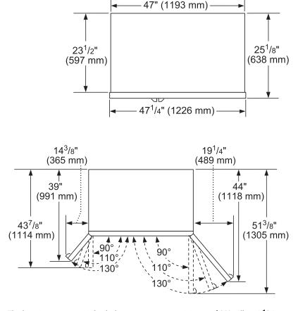
The location must permit both doors to open to a minimum of 90°. Allow 4 1/2" (114 mm) minimum space between the side of the refrigerator and a corner wall.
