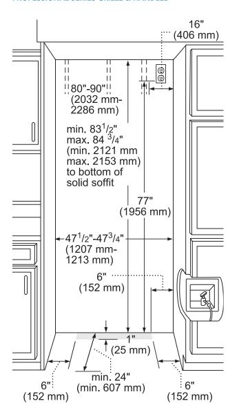
To avoid tipping during use, the solid soffit must be within 1" (25 mm) maximum above the refrigerator. If the solid soffit is higher than 1" (25 mm) or one is not available, then the refrigerator must be braced.
