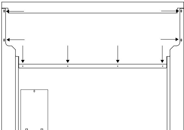
3. Align the back panel of the new accessory with the flanges on the range side panel's right and left rear corners. The backguard is inserted inside the guide channels on the back of the range.
