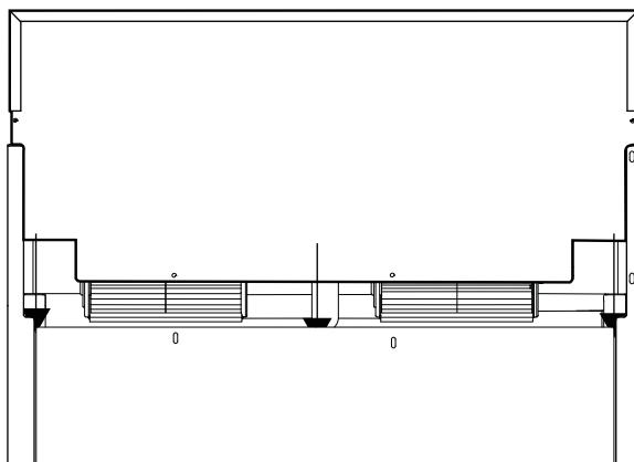
4. Make sure the backguard's front face is outside the flange on the front side of the range.
