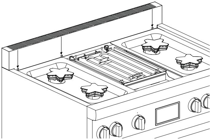
5. Re-install screws removed in Steps 1 and 2.
