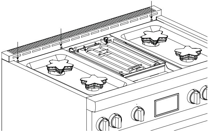
2. Remove the three (3) or four (4) T-20 Torx drill point screws securing the trim to the side panels, and the three (3) or four (4) T-20 Torx drill point screws securing the piece to the back panel. Lift up to fully remove.
