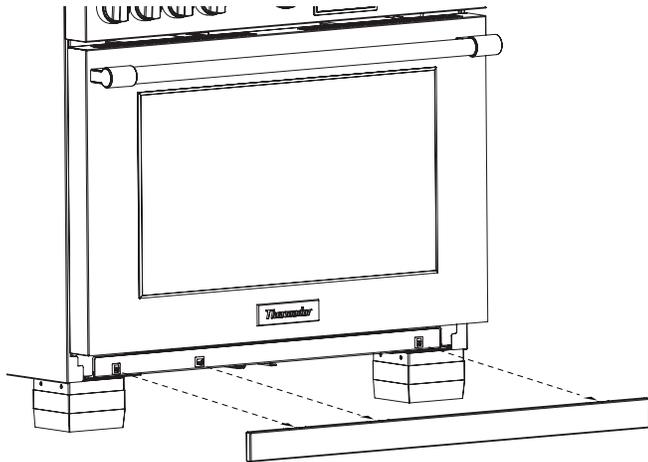
2. Remove the protective plastic coverings from the toe kick and the sliding adjustment panel.
