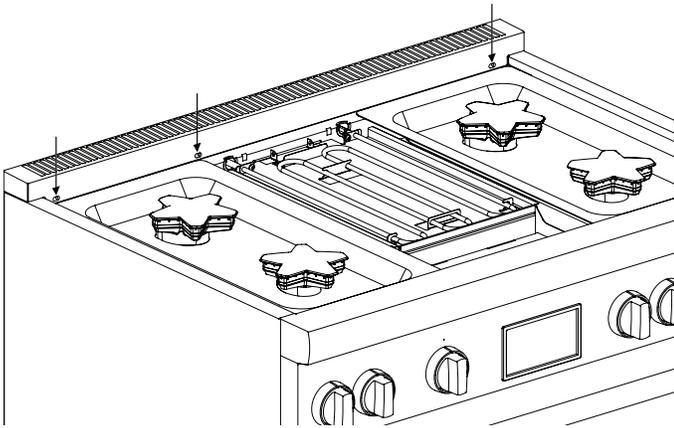
2. Remove the T-20 torx screws securing the trim to the side panels and the back panel. Lift up to fully remove.
