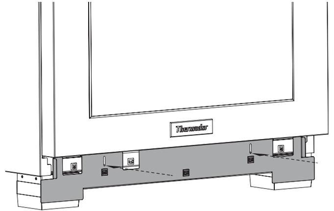
4. Press the toe kick panel into the mounting clips.
