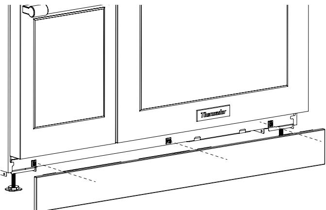
**NOTE:** The mating part has extruded dimples on both sides for which the holes of the toe kick panel should seize. You should feel a definitive snap, letting you know that the part has been installed.
