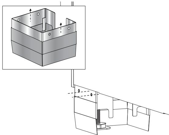
3. Press the toe kick panel into the mounting clips.
