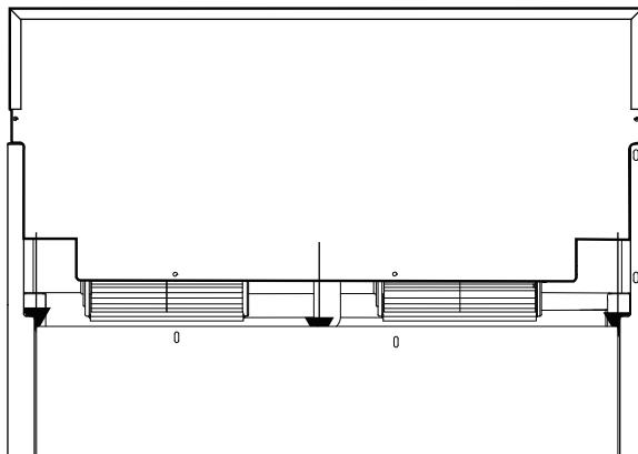
2. The backguard's front face is outside the flange on the front side of the range.
