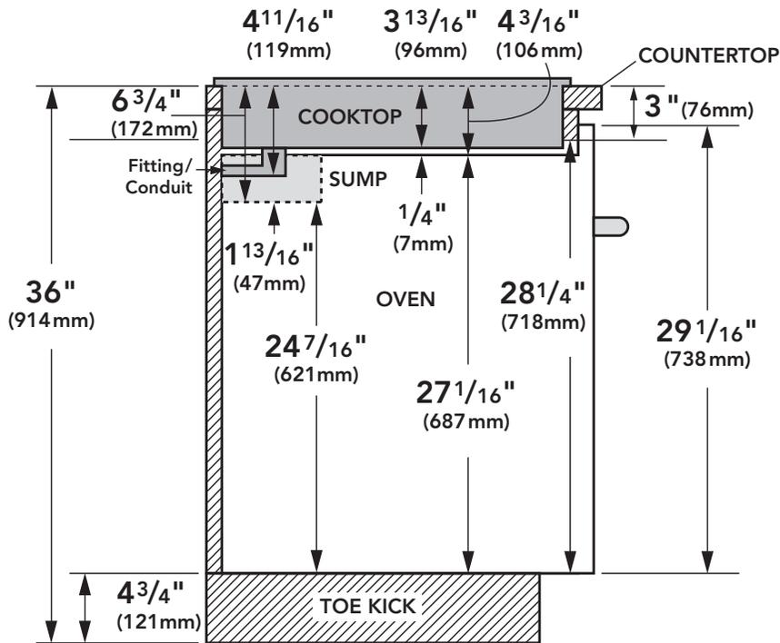
Note: Dimensions based on standard countertop height (36" with 4 3/4" toe kick including base plate).
