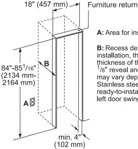
A: Area for installation of power connection.
