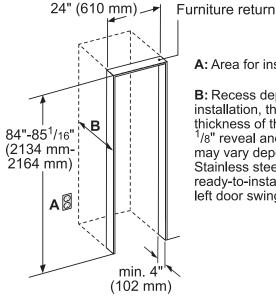
A: Area for installation of power connection.
