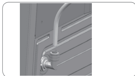
Step 3 ) Connect the PE soft tube.
