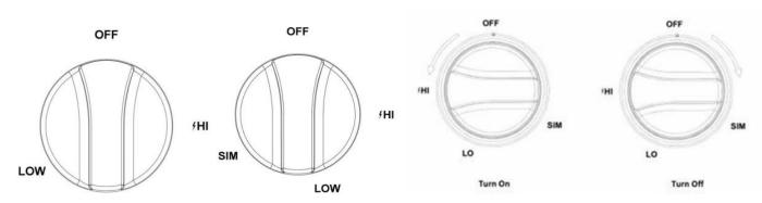
To light the top burners, push and turn the appropriate control knob <u>counterclockwise</u> to the "HI" position. You will hear a clicking noise the sound of the electric spark igniting the burner. Once burner ignition has been achieved, then turn the burner control knob to adjust the desired heat setting.
