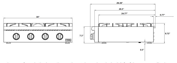
Back Layout from the back panel – Regulator is located on the back left of the range top (back right if you see from the front)
