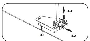
5.Put the Recirculating Kit on corresponding position behind or on the top at range hood, and secure it to the range hood with the matching screw.
