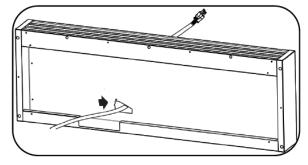
4.Clamp one side of the power cable clip into the power cable hole (4.1) ,fix the power cord to the cable clamp(4.2) ,then fix the cable clamp to the Recirculating Kit.
