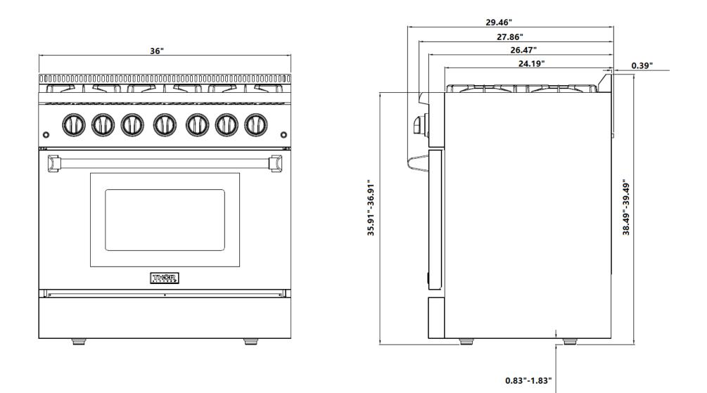
NG: Input Pressure: 7 inches, Output Pressure: 5 inches LP: Input Pressure: 11 inches Output Pressure: 10 inches **Regulator Location: Inside the kick Panel – Bottom Right** Size of Regulator: ½ inch
