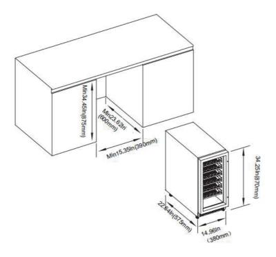
Attention: The ventilator should not be covered, or it will cause unpredictable breakdown; the fan and the return-airway should not be covered, too, or it will cause the temperature of the wine cooler couldn't reach the setting temperature, and the temperature of the cabinet is uneven.
