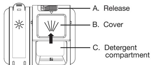
Close the detergent dispenser by sliding cover (B) over detergent compartment (C). Open the detergent dispenser by sliding release (A) to the left and the cover (B) will automatically slide open.
