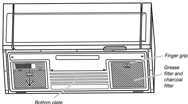
2. Clean the grease filter monthly, or replace with a new grease filter if necessary.
