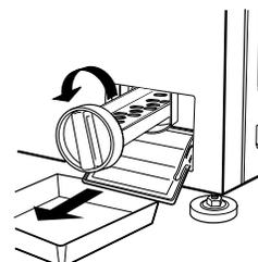
3. Clean the filter with a soft brush under running water until all residue is removed.
