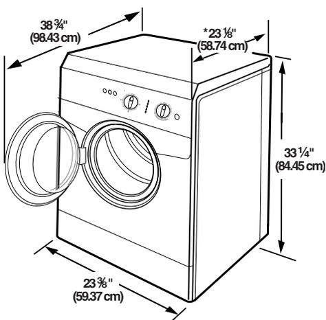
\*Most installations require a minimum of 4" (10.16 cm) clearance behind the washer for drain hose clearance. See “Drain System.”
