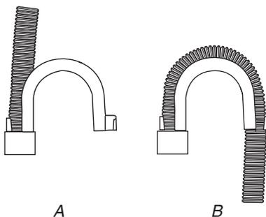
A. Snap either end of the U-shaped hose form to the drain hose at the point where the corrugation begins.
