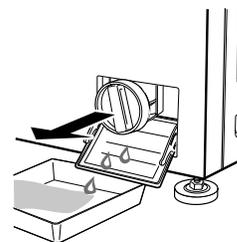
2. Remove the filter by rotating it a half-turn counterclockwise and pulling outward.
