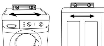
4. If the washer is not level, prop up the front of the washer with the wood block and adjust the feet up or down as necessary. If the washer is against a wall, move the washer out slightly before tipping back. Repeat this step until washer is level.
