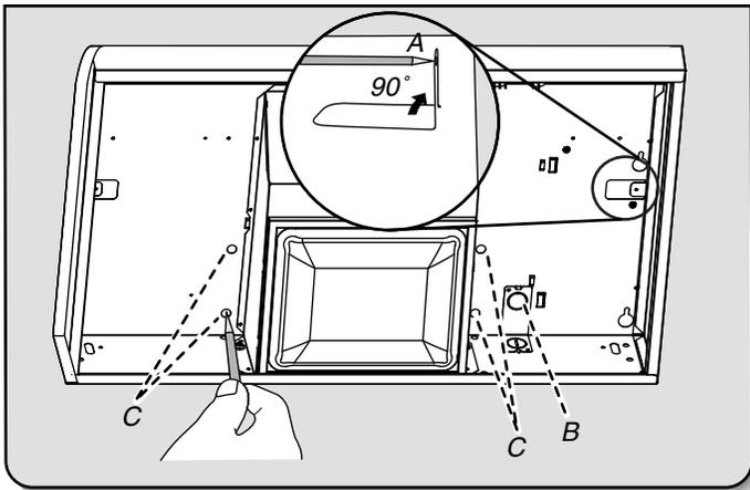
Hold the range hood firmly in place with one hand and bend each mounting tab (A) upward approximately 90°.
