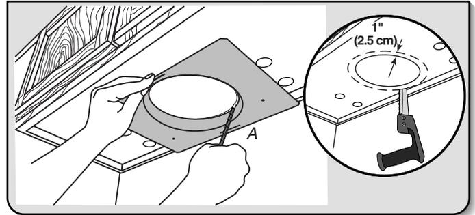
■ Using the 7" (17.8 cm) round vent mounting plate, draw the vent opening outline on the underside of the cabinet:
