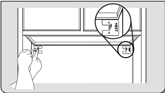
Align the exterior edge of the mounting brackets with the exterior edges of the upper cabinet.
